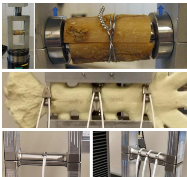
Resim 1. Mechanisms used for tested samples - Double loop wire, Dual Polymer Cable x3, Ortholox ® UHMWPE Double Wrap, Ortholox ® UHMWPE Single Wrap x3 systems mounted on test mechanisms
